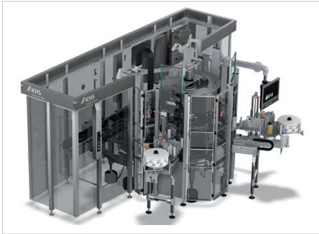
The Innoket Neo can label up to 35,000 full or empty cans in all standard sizes per hour. © KHS
