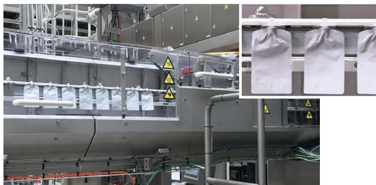
The JBT AsepFlex Linear Pouch Filler has a capacity of 500 ppm or 30,000 pouches per hour. © JBT
